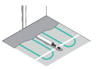
When positioning the sensor try to avoid hot water pipes in the floor or any draughty places such as external doorways as this may affect the thermostat. If required, the sensor lead can be extended using twin-flex cable.
